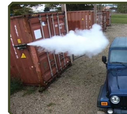
Image: Omnihammer Sim detonated remotely, attached with magnetic caddy
